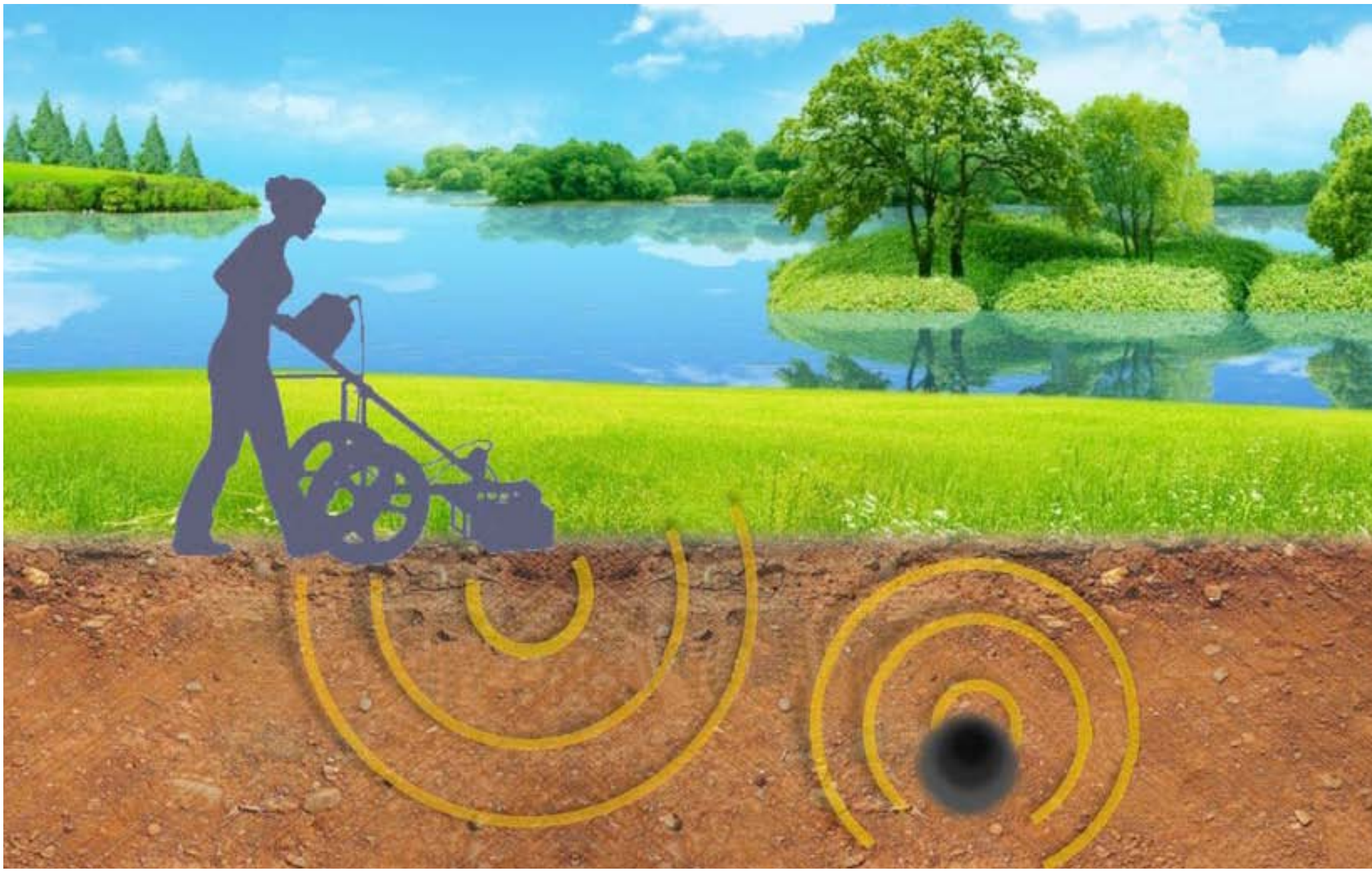
Detecting buried objects – electromagnetic wave propagation from a GPR
